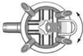
The Classic 300 E clawpiece with narrower positioning of the short milk tube connections for the rear quarters
